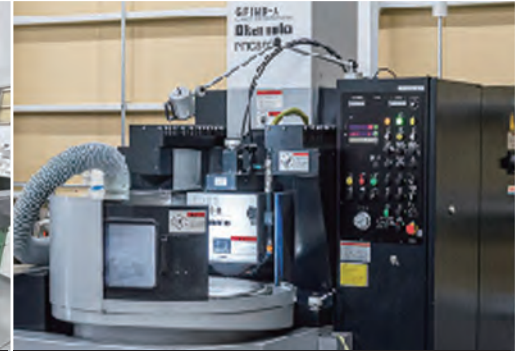
Horizontal axis rotary grinding machine \phi 800
