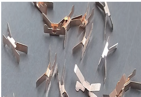
Ultra-thin Micro Parts t=0.07\text{mm}
